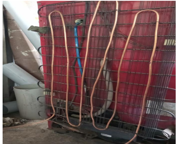
Fig -3.1: Winding of copper coil around condenser
